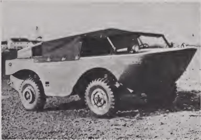
FIGURE 18. 1942 model of "Aquacheetah" representing "ground-up" design of 3/4-ton, 4x4 amphibian built by Amphibian Car Corp.
